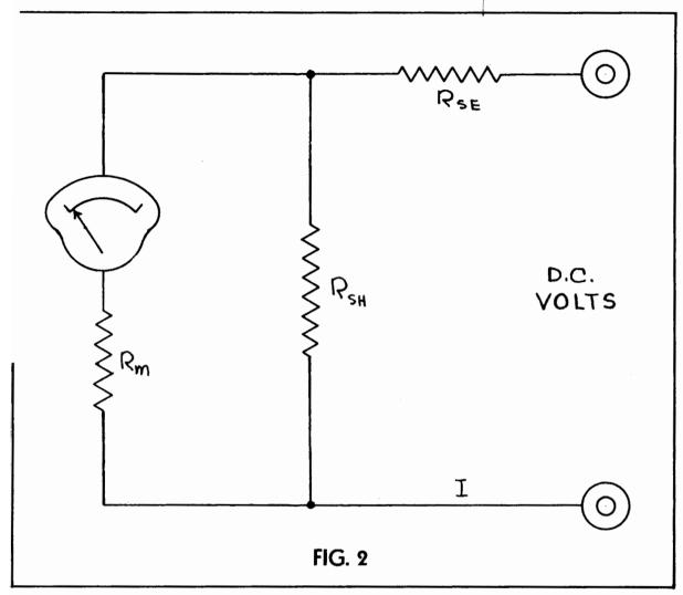
shunt resistance portion of R, (i) is the current through the meter, and I is the current being measured.
