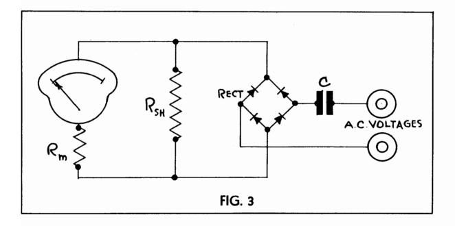
still remain at 1 ma. for full scale deflection, with a 1000 ohms per volt sensitivity.
