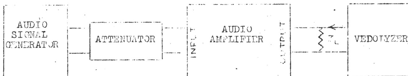
Fig. 1-5 SET-UP FOR FREQUENCY RUN OF AN AUDIO AMPLIFIER
